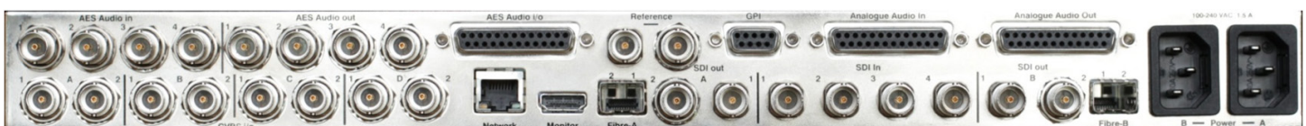
Rear panel shows MC2000 with CVBS option fitted.
